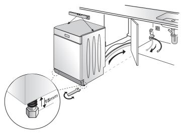
When the appliance is correctly levelled, the door will not catch on the inner liner on either side of the cabinet.
